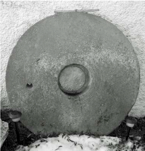
Figure 2. Baldernock Mill runner stone viewed from the underside. Note the cross section of the eye and the circular grooves around it. The ruler on top of the stone is 457 mm (18 in) long.
