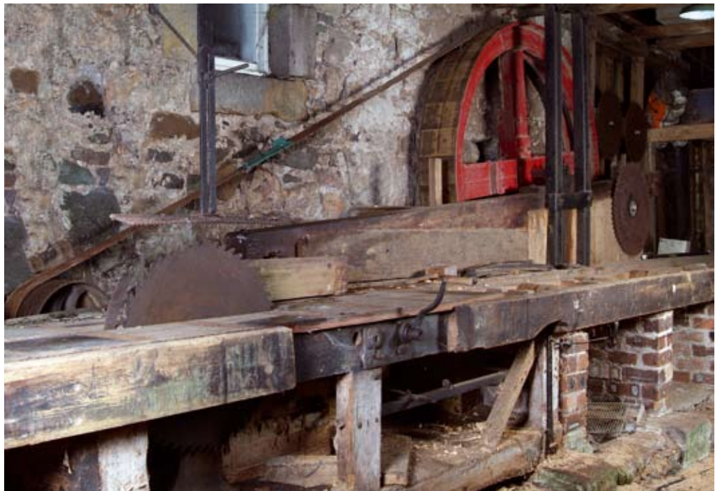
Figure 4. The saw bench in the saw mill. The large red fly wheel, driven by the shaft with the bevel gear, drives the belt to power the saw blade (left) (photo by Les Hill)
