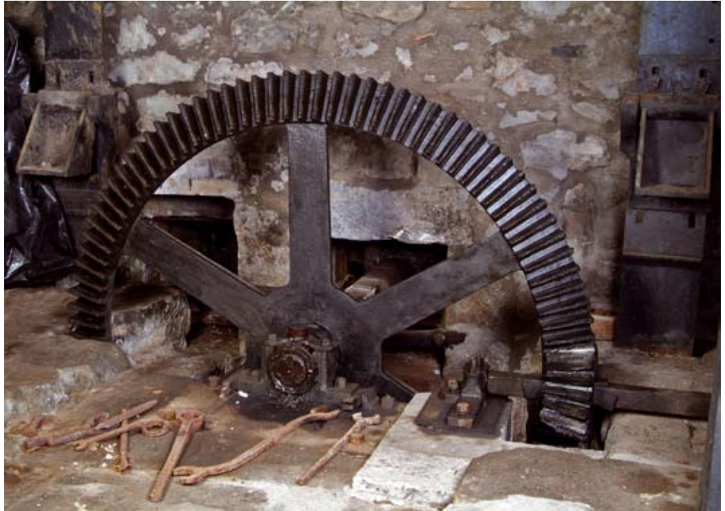
Figure 3. The drive shaft from the mill wheel with large geared pit wheel that drives the fly wheel in the saw mill via the bevel gear and shaft to the right (photo by Les Hill)
